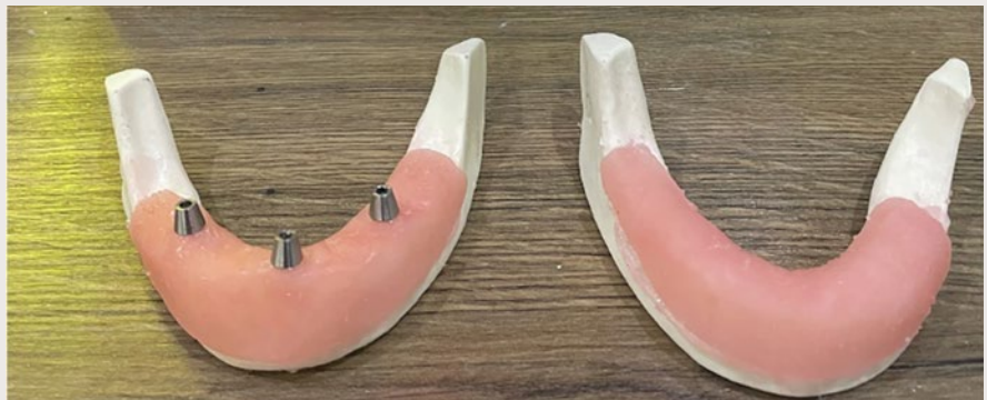
Figure 3: Artificial Bone Model Type A - With Novel Two Part Screws and Type B - Without screws
